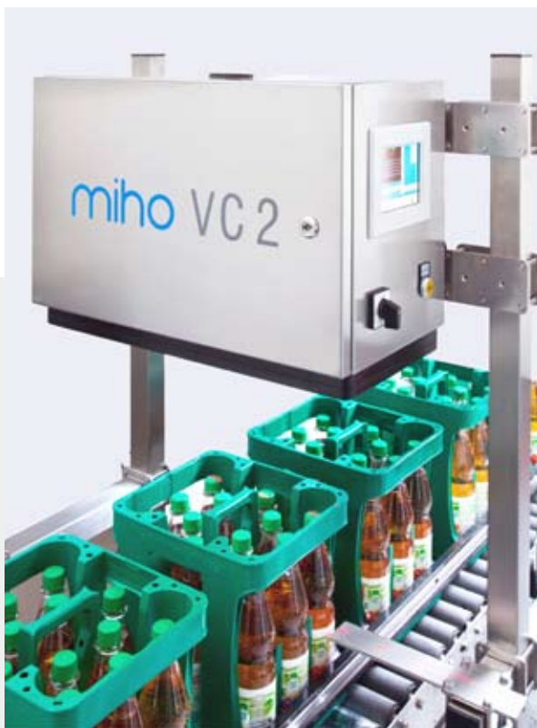
Examples of innovative miho inspection processes: Full crate inspection using a line laser (subject to patent)
