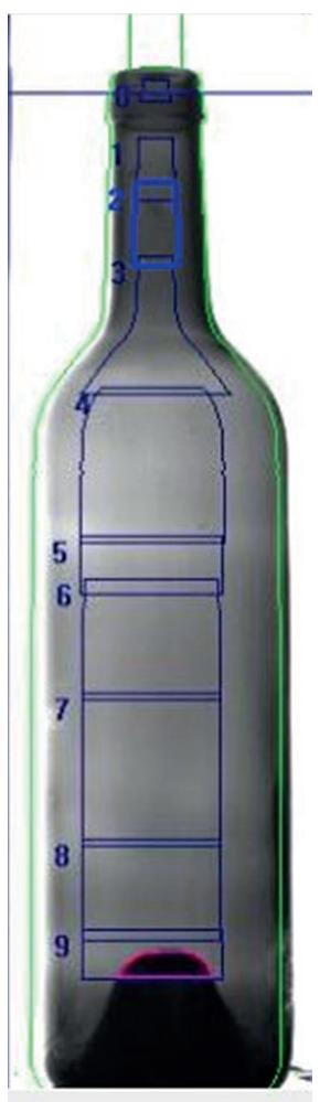
The bottle with the lower dome is set to be a "good" bottle. Thanks to the flexibility of the inspection software miho VIDIOS©, an inspection zone no.9 detects the bottle with the large dome as to be rejected. As a result, a sorting by the height of the dome is reliably given.
