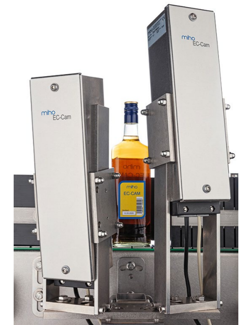
Figure 4: Full bottle inspection of non-cylindrical containers.
