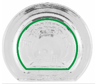
Non-cylindrical bottle with embossing on the base. Unrestricted inspection in the green area
