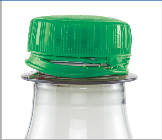
Broken safety ring
