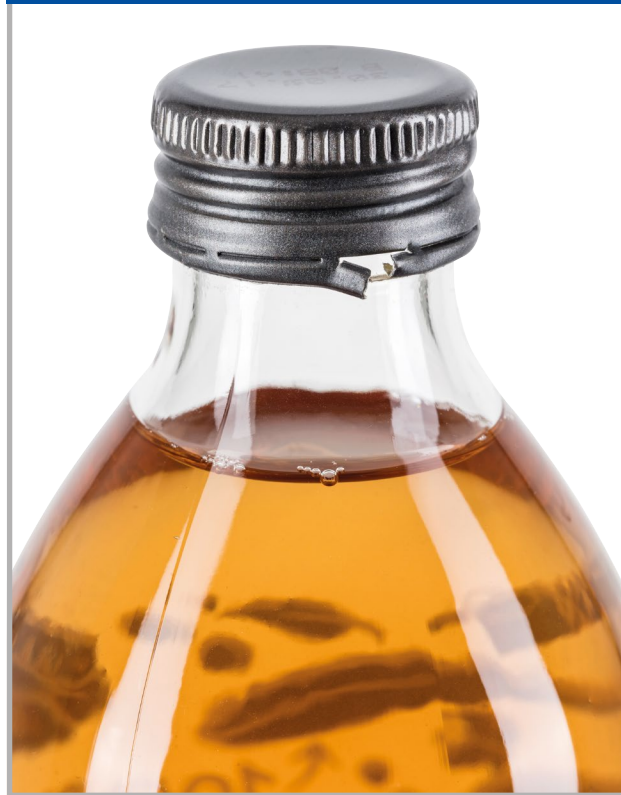
360° check: broken safety ring
