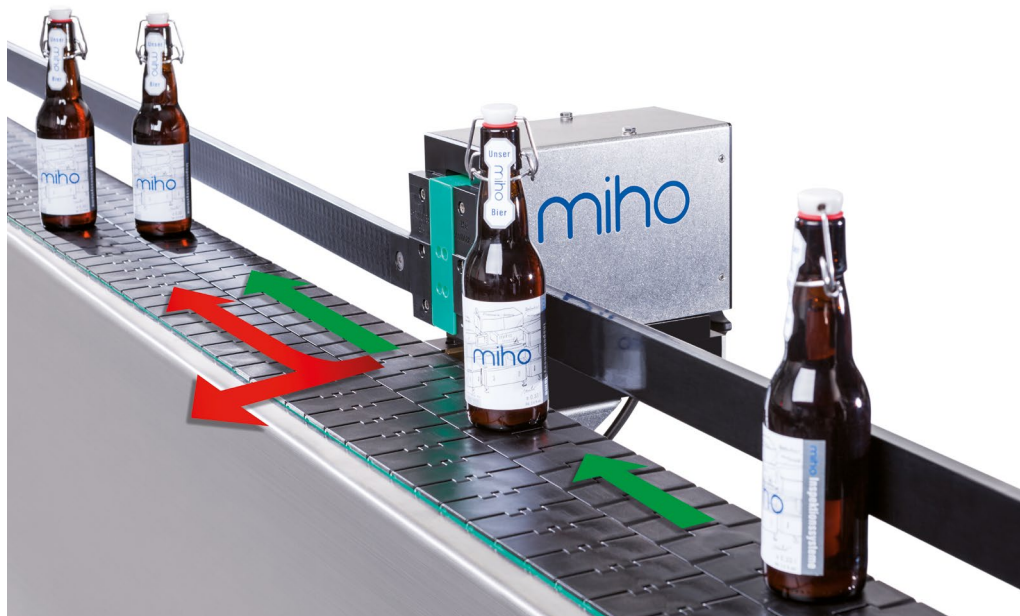
miho HSPM: Multiway rejection (red arrows), depending on the kind of container defect
