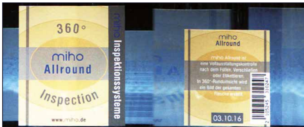
The four individual images of the side cameras (top) and the completely processed and rectified overall image of the bottle (bottom)
