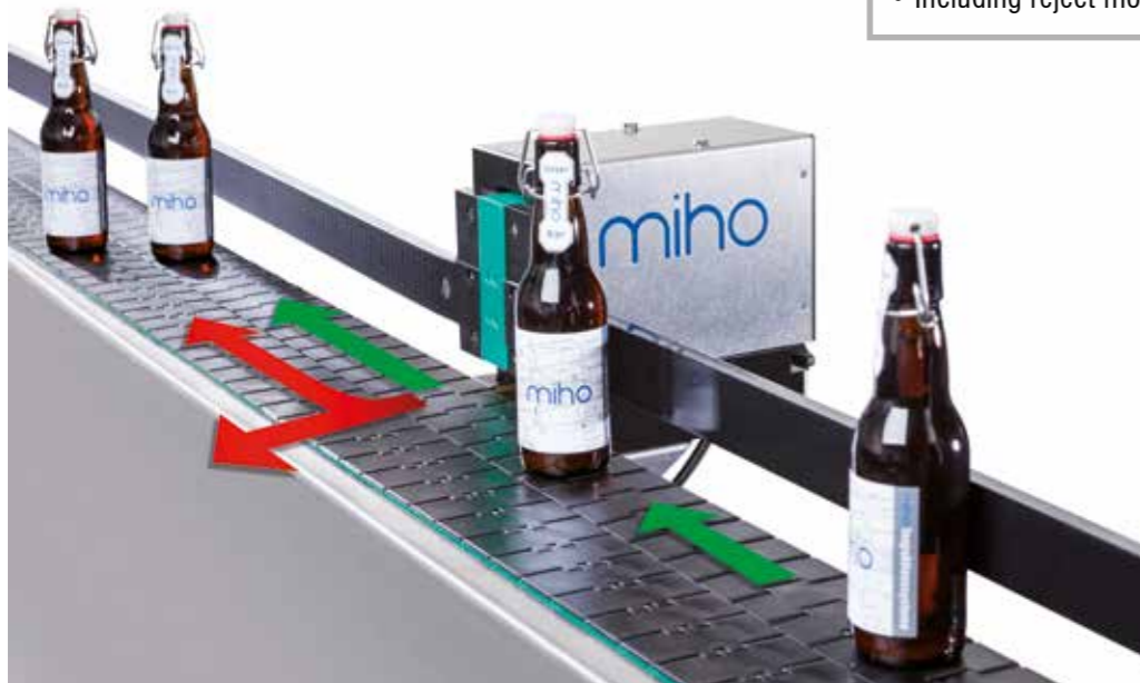
miho HSPM: multiple rejection (red arrows), depending on the type of bottle defect
